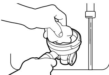
The filter holder should be cleaned to remove the greasy coffee residues that can negatively affect the taste of your espresso. Wash the exterior part of the steam wand with a damp cloth and release a little steam to remove any milk residues from inside the tube, as these could obstruct the steam output, making it more difficult to froth milk properly.
