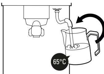
Insert the wand all the way down and tilt the jug to create a vortex. Heat the milk to the desired temperature, without exceeding 65°C. *Close the steam.*
